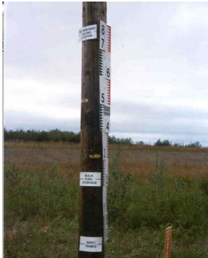
Figure 5-9b City of Holy Cross Flood Gauge Side View (USACE 2011)
