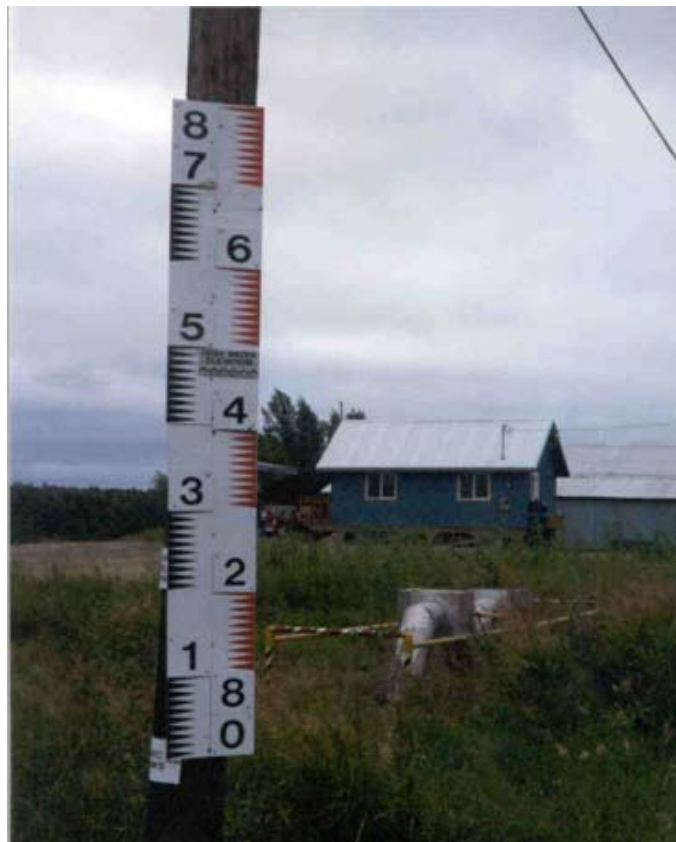
Figure 5-9a City of Holy Cross Flood Gauge (USACE 2011)
